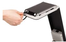
Insert the USB Cable at the Docking Platform into the Compact 6 HD Speech USB port to charge the Compact 6 HD Speech and to connect the speaker.
